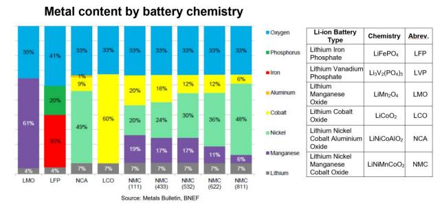
Figure 3. Illustration of commodity content of various lithium-ion batteries.
