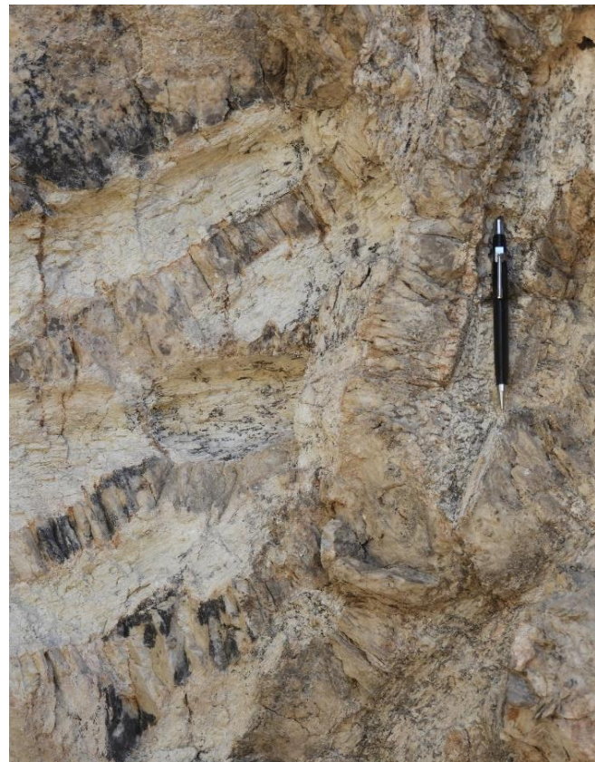
Coarse Li Spodumene Crystals, Previously Explored for and Exploited in Small-Scale Workings
